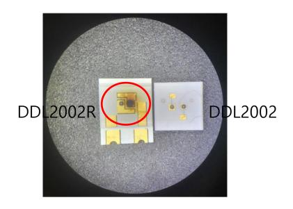
DDL2002R was burnt out @200mA high DC continuous current within 1min, while DDL2002 was still OK over 10min.
